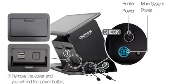
2 Connect the peripheral cables to I/O ports on demand.
