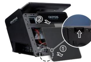
1 After unlinking the hook of back cover on the bottom of main system and
