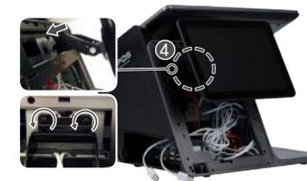
4 Install a dual monitor and fasten the screws.
