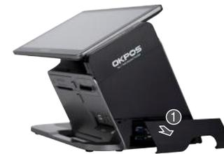
1 Open and pull up the cable cover for detaching.
